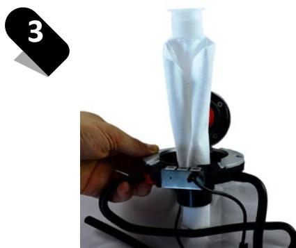
Push the adapter with two thumbs as deep as necessary just to allow the correct closing of the lid.
