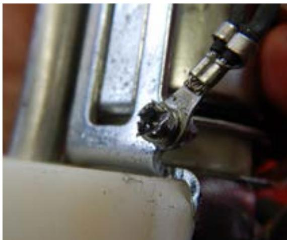
Detach the ground wire from the fuel pump. Hopefully you will find that the screw is not too tight and can be removed easily and without damage, unlike this one on the photo above.
