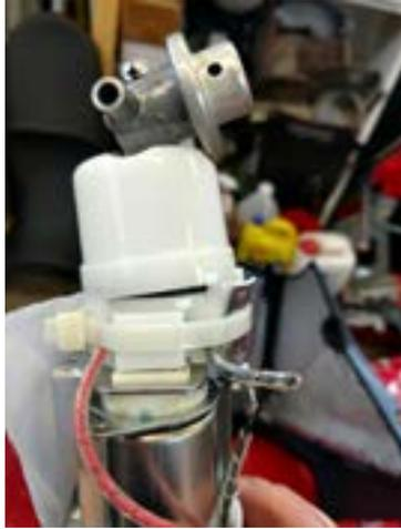
While closing back the upper part, install, always with a drop of engine fresh oil, the provided new o-ring. Close it properly paying attention to check many times the correct position both of the two halves and of the assembly on top of the fuel pump itself.
