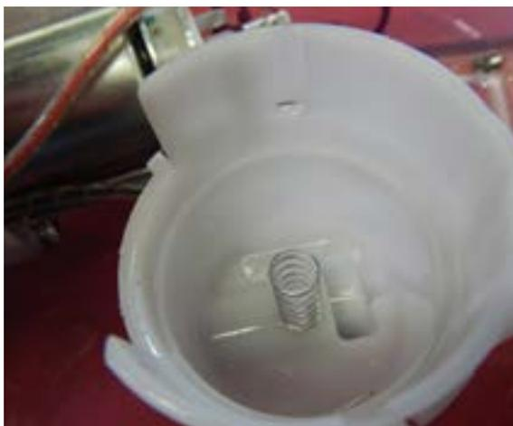
Remove and discard the spring which holds in place the OEM paper filter. The mini o-ring in the filter can be used as a replacement for the fuel quickdisconnect.
