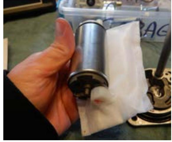
Press the plastic filter neck of the Godzilla filter onto the intake at the base of the fuel pump.
