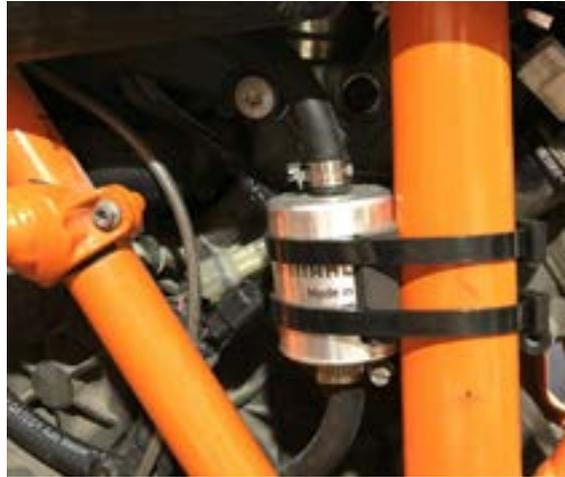
Once all parts are back in place, DO NOT switch the engine at once. Prime the system doing 5 times the std check, rotate the key, do the ignition check and switch off, with each action you may notice a different sound from the pump, sign that it is bleeding out the air, on the 6th turn of the key, start the engine. You're GOOD TO GO.
