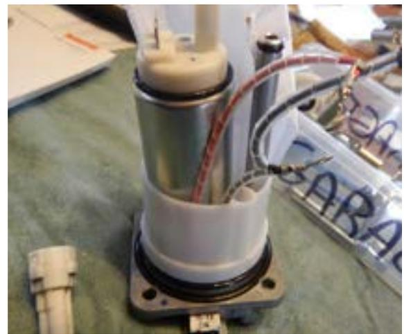
Replace the lower white plastic housing, taking care not to pinch the filter media or electrical wires. Reassemble the upper parts of the plastic housing, attach the ground wire and reinstall the fuel pump.
