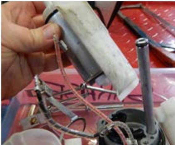
Lift the fuel pump out of the dark plastic base. The OEM filter is press fitted onto the base of the pump; remove and discard the OEM filter.
