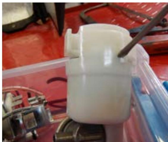
The OEM paper filter is located inside the plastic head. Use a small flat head screw driver to gently depress the plastic tabs shown in order to remove the lower half of the plastic unit and expose the paper filter.
