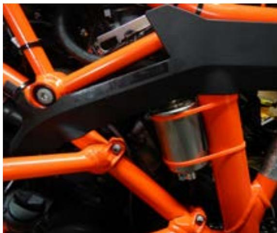
We can provide without extra costs a larger unit to be mounted on the frame, easier to access and to change for servicing, as always position it vertical with the "out" on top.
