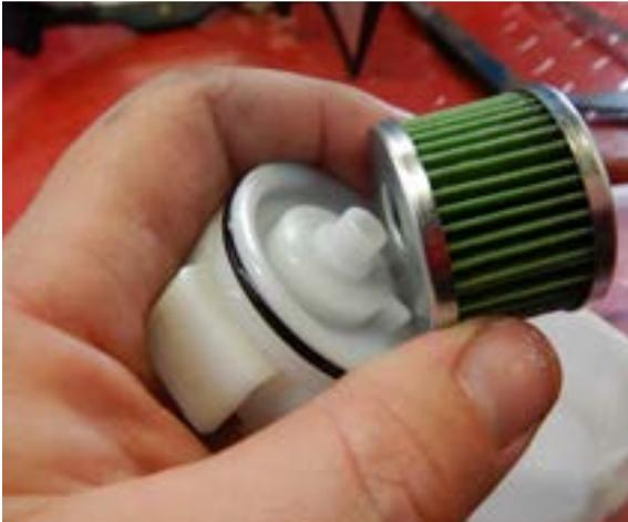
The Fuel System NEEDS A MAIN FILTER, either you will wash and re-use the paper original one, or you MUST INSTALL an In-Line or Out of Tank Fuel filter. If you install the latter, the paper filter will be disposed of system. Remove and discard the OEM filter.
