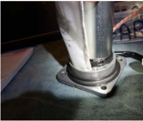
Ensure that the Godzilla filter is aligned parallel to the fuel pump so that the filter will fit easily back inside the housing. You may need to rotate the plastic filter neck so that the filter body is positioned correctly, following the red arrow designed on the Godzilla neck.
