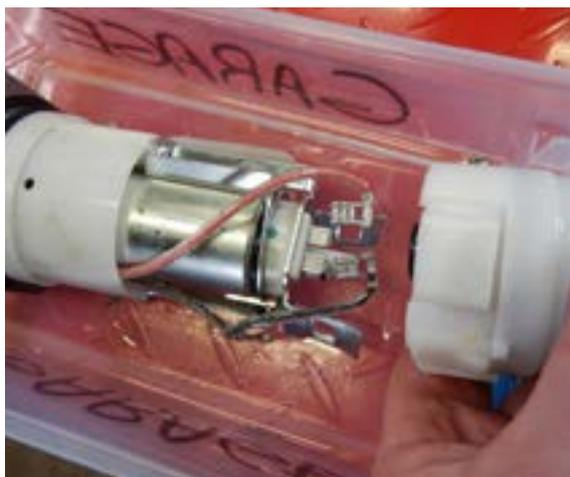
Once the fuel pump is completely removed from the tank, remove the plastic head of the fuel pump. There are two plastic tabs which need to be depressed before the plastic head can be gently removed.
