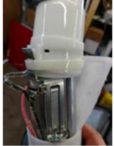
Failing to do so, if the assembly is not correctly repositioned, it will eventually pop open again due to fuel pressure. Install the provided large cable tie to push down the two metal lips and hold the whole assembly into position.
