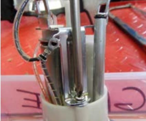
Remove the two screws which hold the fuel pump into the base of the fuel pump housing. Lift off the lower white plastic housing.
